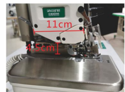
机头仅11cm宽，高4.5cm，超大操作空间 The head is only 11cm wide and 4.5cm high, with large operation space
